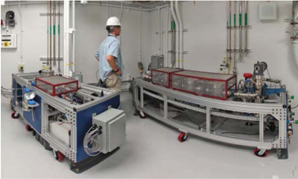
Figure 45. The RAGS hardware at the NIF. Directly after a shot, the gaseous products inside the target chamber are pumped out and into RAGS, where unwanted species are filtered out from the gas (this happens in the right cart shown in the figure). The noble gases are subsequently frozen and analyzed to quantify the number of nuclear reactions that occurred in an implosion. This happens in the left cart shown in the figure. Reprinted from [222], with the permission of AIP Publishing.
