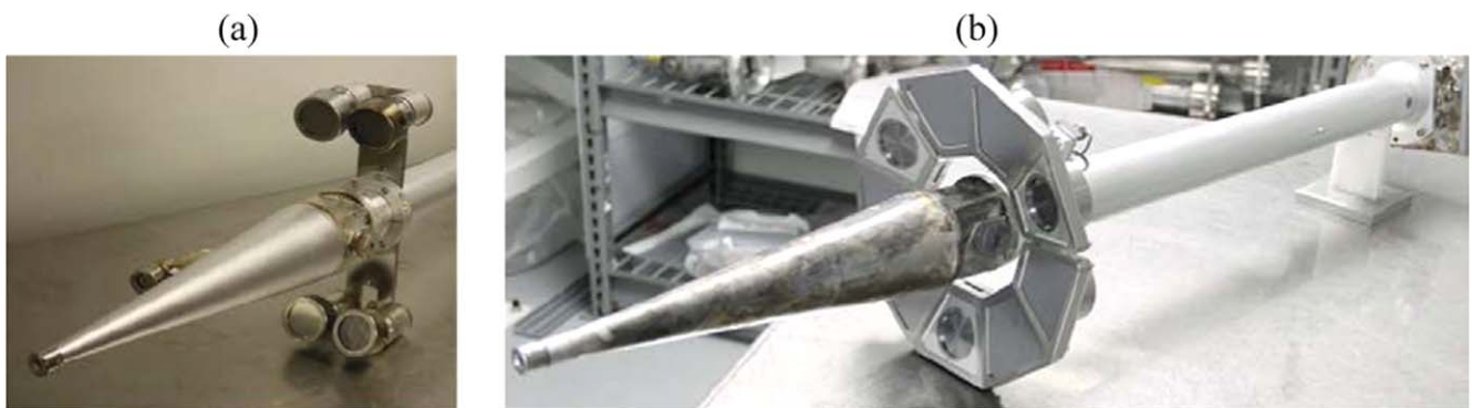
Figure 46. (a) Pictures of the SRC systems. (a) The SRC with a 2 inch diameter disc of either tantalum, vanadium or carbon. Up to four SRC systems can be fielded on one DIM. Reprinted from [224], with the permission of AIP Publishing. (b) The Vast Area Detector for Experimental Radiochemistry (VADER) system for solid radiochemistry collection.
